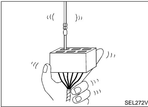
4. While moving the connector, check whether the male terminal can be easily inserted or not.
