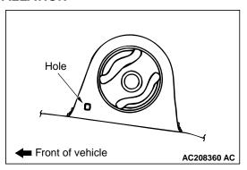
Install the engine roll stopper bracket so that its hole points towards the front side of the vehicle.
