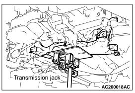
Retain the crossmember with a transmission jack, and then remove the crossmember mounting bolt.
