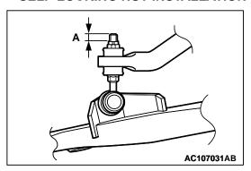
Tighten the self-locking nut until the stabilizer link thread part protruding length meets the standard value.
