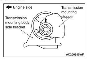
Install the transmission mounting stopper so that its arrow points upward.
