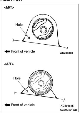
Install the engine roll stopper bracket so that its hole points towards the front side of the vehicle.
