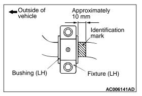
Align the stabilizer bar identification mark with the right end of the bushing (LH).
